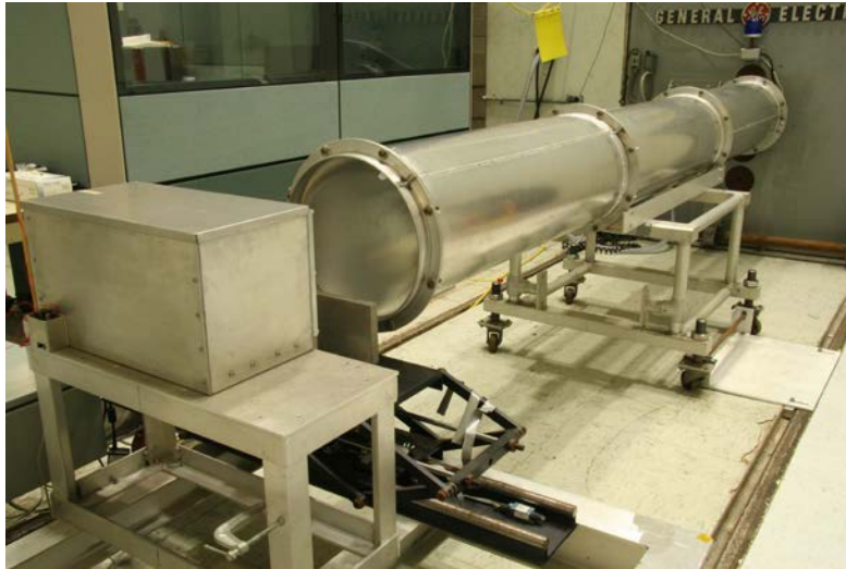
Fig. 1 Thermal Column with removable beam extender
