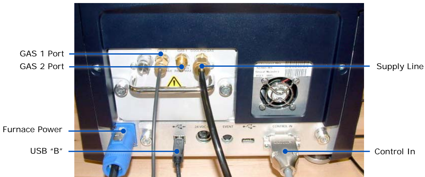
Figure 4 Discovery DSC Rear Panel Connections
